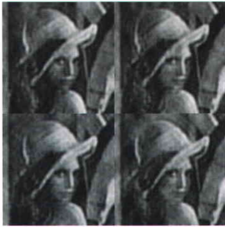
Figure 11: Four produced sub-images of the extracted watermarks, w_1 , w_2 , w_3 and w_4 after rescaling and inverse DCT.
