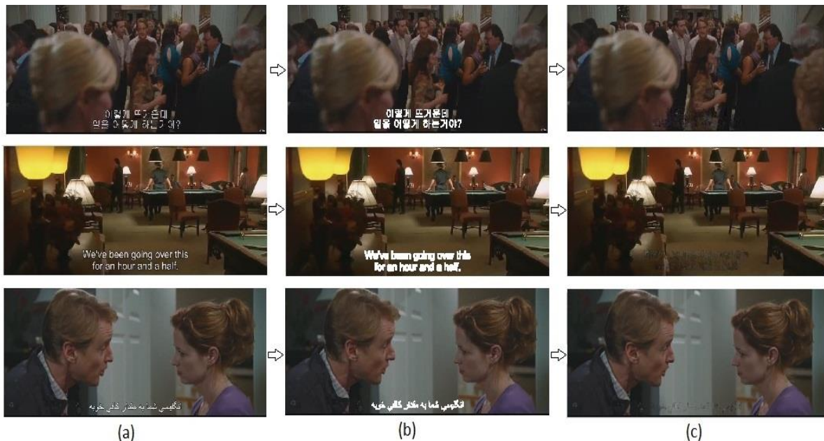
Fig. 12. The results of text localization, extraction and inpainting algorithms (a) original images, (b) the extracted texts, (c) the reconstructed images after applying the proposed text extraction and inpainting algorithm.
