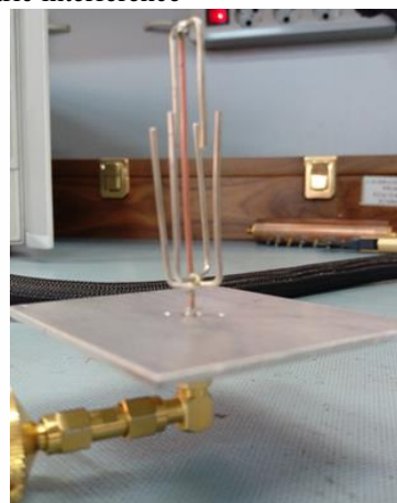
Figure 2. Fabricated multi-band monopole antenna.
