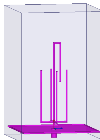
Figure 4. Simulation of the proposed antenna by using HFSS.
