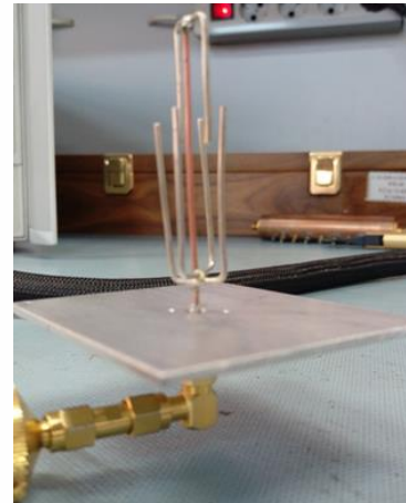
Figure 2. Fabricated multi-band monopole antenna.
