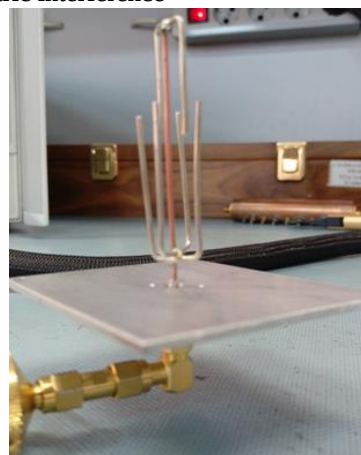
Figure 2. Fabricated multi-band monopole antenna.
