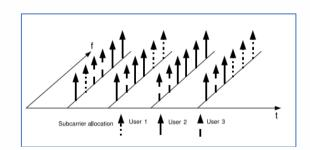
Principle of OFDMA sub-carrier allocation [4]..
