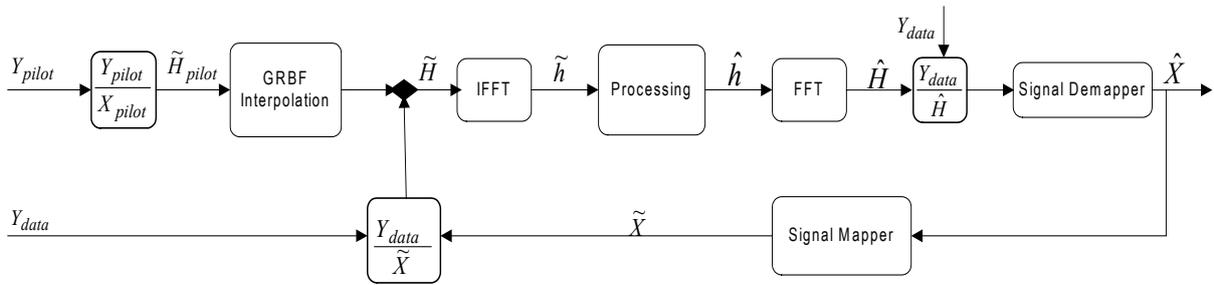
Figure 5. Channel Estimation and Detection structure block diagram for OFDM system.
