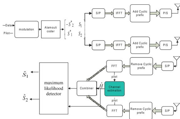
Figure 2. Alamouti coded OFDM transceiver block diagram.
