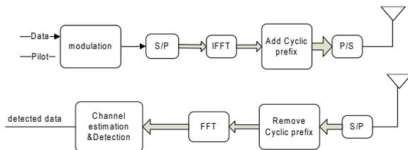
Figure 1. OFDM transceiver block diagram.
