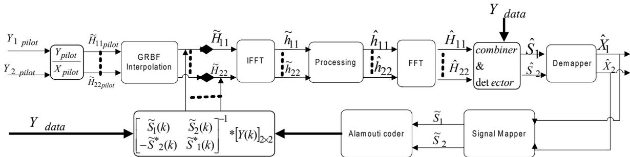
Figure 6. Channel Estimation and Detection structure block diagram.
