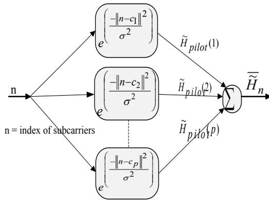
Figure 7. GRBFN structure for Channel Estimation.
