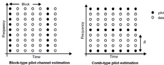
Figure 3. Two Basic Types of Pilot Arrangement for OFDM Channel Estimations [9].
