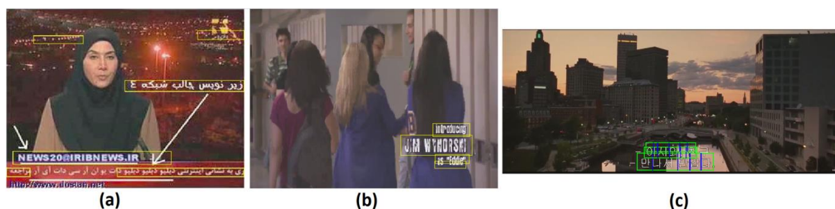
Fig. 14. Source of errors for the proposed text localization algorithm. (a) Error of text verification stage, (b) error because of low contrast texts and holes in texts and (c) error because of separating nearby text areas using block split and merging algorithm.
