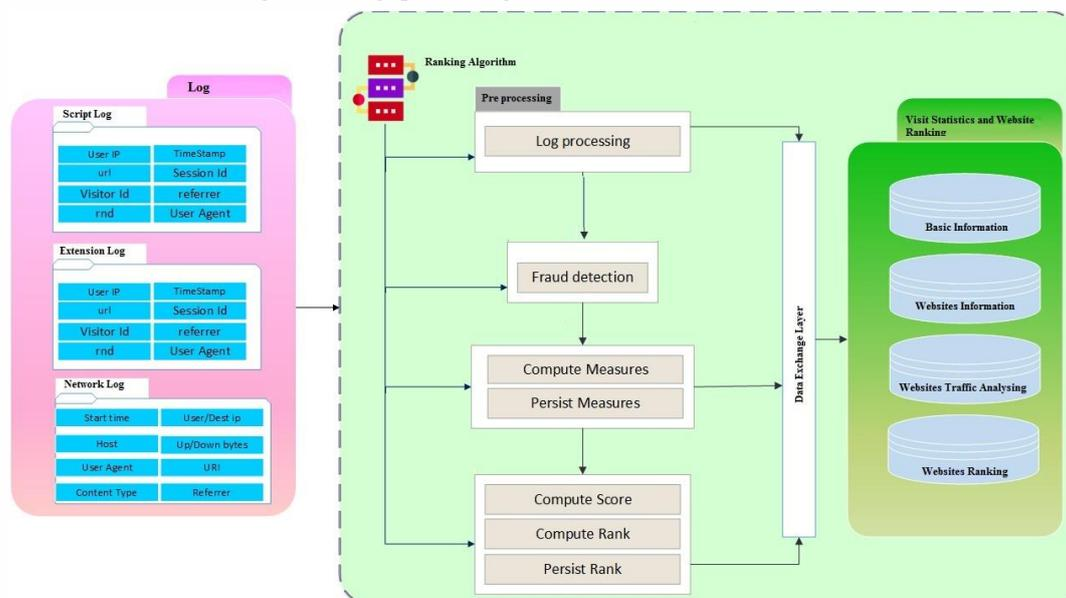
Figure 2. Architecture of web domain ranking and traffic analyzing subsystem.
