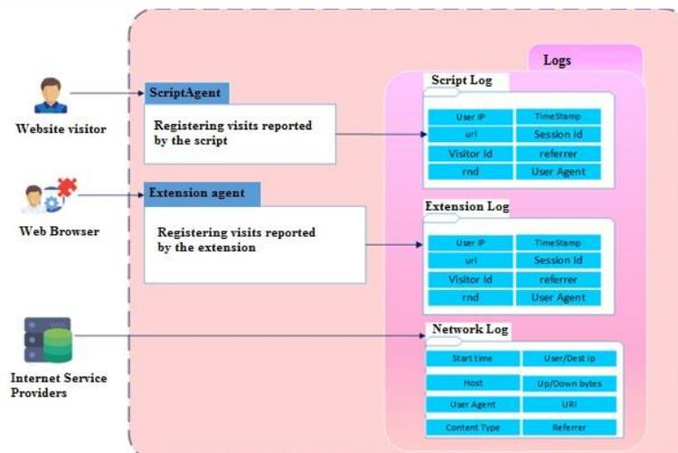
Figure 1. Architecture of Traffic Data Collection Subsystem.
