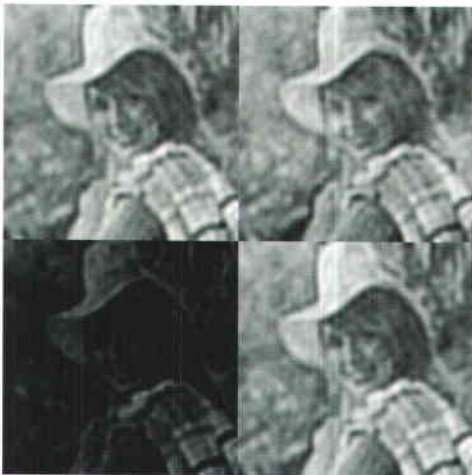
Figure 19: Four produced sub-images of the extracted watermarks, w_1 , w_2 , w_3 and w_4 after rescaling and inverse DCT.
