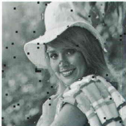
Figure 23: The reconstructed image after error concealment of Fig. 18, by the method given in [6]; PSNR= 26.4437.
