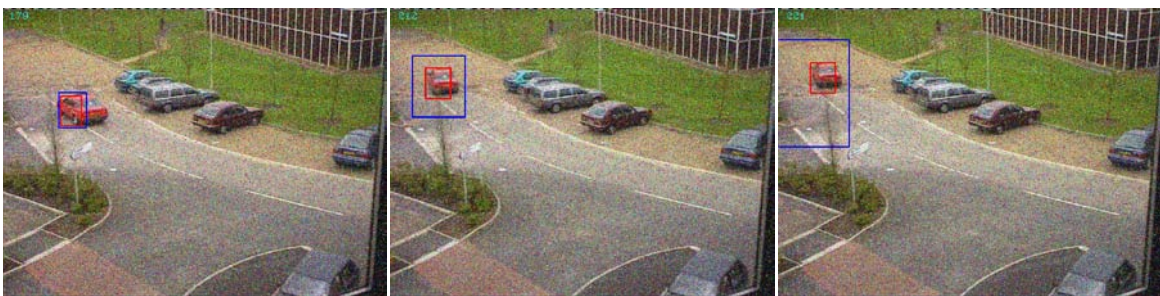
Figure 5. Traditional CAMShift(blue rectangle) fails in tracking the target in the presence 20% noise, while the improved CAMShift tracks the target successfully (red rectangle).
