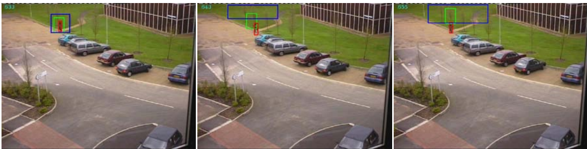
Figure 4. Traditional CAMShift(blue rectangle) and mean-shift(green rectangle) fail in tracking the target due to poor search window initialization, while the improved CAMShift tracks the target successfully (red rectangle). Search widow is initialized several frames before the first shown frame.
