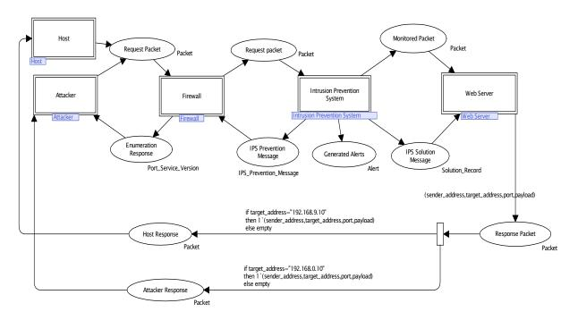
Figure 3. The model created for the network of Figure 2
