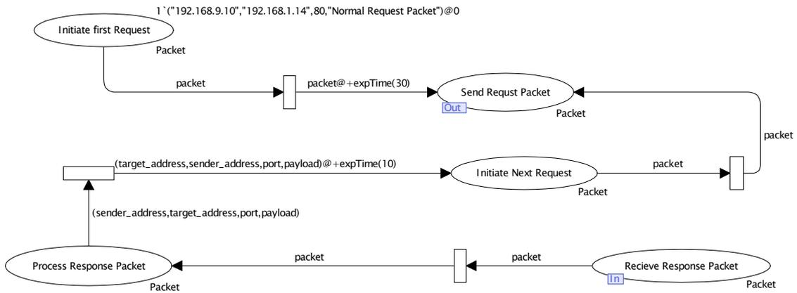
Figure 4. The CPN sub-model for the host
