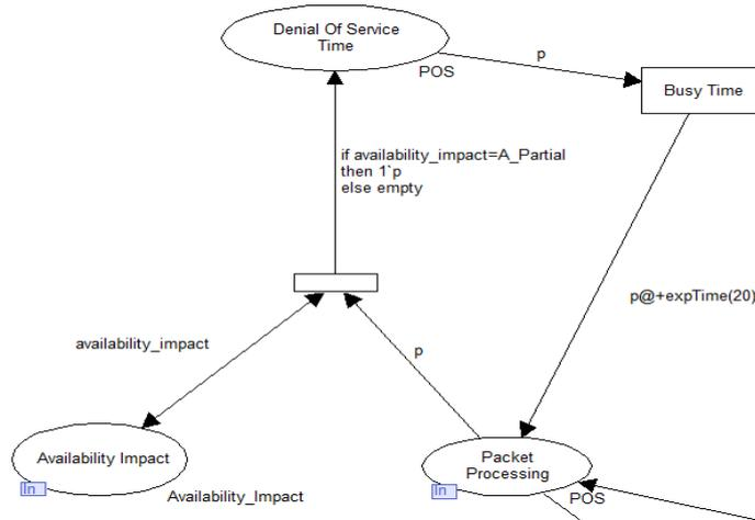
Figure 18. Modeled ON/OFF process for partial availability impact
