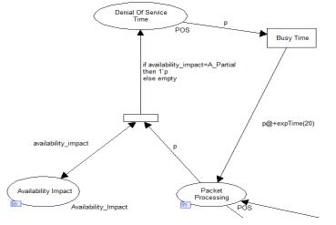
Figure 18. Modeled ON/OFF process for partial availability impact
