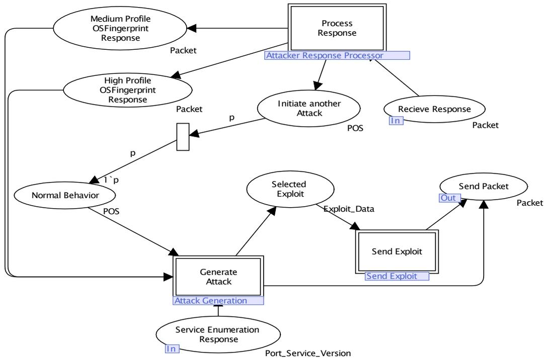
Figure 7. High-level model of attacker
