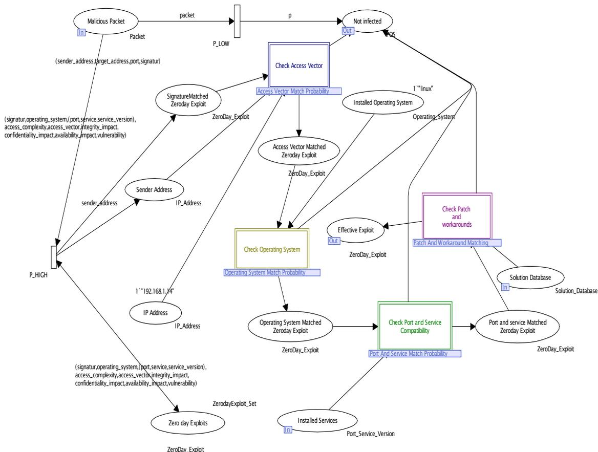
Figure 15. Exploit infiltration success probability model
